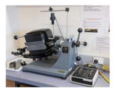
SG Frantz LB-1 magnetic susceptibility separator utilising paramagnetic and diamagnetic properties of minerals.
