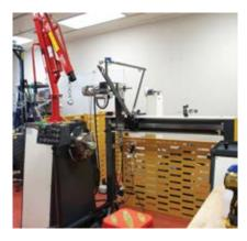
Capable of winding coils or coil assemblies up to 1 m diameter and 1.2 m long. Can wind LTS, HTS, or copper wire up to two-in-hand with 5 kg tension.
