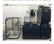
lon chromatography system used in the ice core laboratory.
