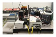
World-leading measurement rig capable of PLQE measurement at any wavelength excitation. 300–1100 nm.
