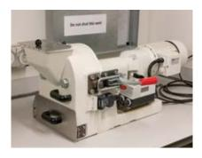
This disk mill is used for efficient fine grinding of hard-brittle to medium-hard solids. Features include automatic locking of the collecting vessel and grinding chamber, and motor-driven grinding gap adjustment with digital gap display. Ideal for medium particle sizes in the areas of mining and metallurgy, ceramics industry, rocks and soils, glass industry, and soil research.
