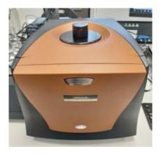
Differential scanning calorimeter for the determination of melting temperature of biomolecules.
