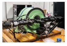
This ellipsometer operates by polarisation modulation with an elasto-optic modulator. A wide wavelength range (196 to 2000 nm) can be used with this instrument.
