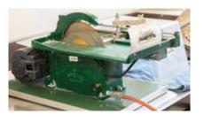
Lapidiary 250 mm diameter diamond saw for trimming small rock samples. Hand feed or automatic drive.
