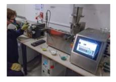
This a laboratory plastic extrusion machine, used for trialling/researching different plastic mixes and recycling scenarios, with the suite of FDM 3D printers on site—in particular the Big Rep. This enables an end-to-end product recycling or specialist resin 'mixes' for research.
