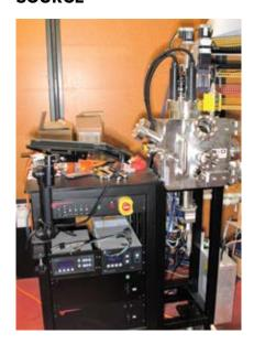
Multi-target thin film high vacuum PLD system with heated substrate stage up to 900°C.
