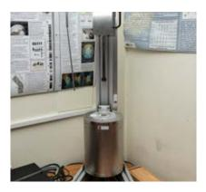
The Triaxe Magnetometer allows for the rapid estimation of palaeointensities from volcanic and fired archaeomagnetic samples.
