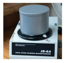
For measurement of the remanent magnetisation of rock, sediment, or archaeomagnetic samples for palaeomagnetic studies. Complementary laboratory equipment for thermal demagnetisation, alternating field demagnetisation, magnetic susceptibility studies, including variation with temperature, and isothermal remanent magnetisation studies.
