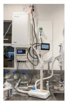
Supply purified Milli-Q water for laboratory use.
