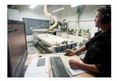
Techno Full Sheet (LC 48" x 96") flatbed CNC router. Setup uses Rhino Cam for toolpaths.
