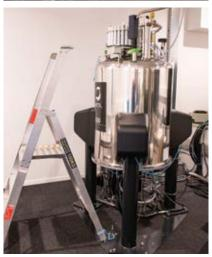
Three JEOL machines—3-Channel 500 MHz Nuclear Magnetic Resonance Spectrometer. 2-Channel 500 MHz Nuclear Magnetic Resonance Spectrometer type JNM-ECZ500S for routine analyses aimed towards 24/7 routine analyses. 600 MHz Nuclear Magnetic Resonance Spectrometer type JNM-ECZ600R.
