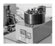
Alpha dose source used for the luminescence dating of samples and materials.
