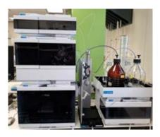
Separation and purification of chemical compounds using UV detection.
