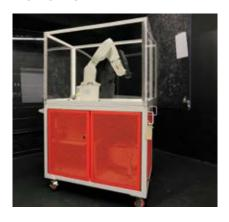
ABB Robotic Arm (small mobile IRB 1200-7/0.7 m). Used largely for small-scale testing and demonstrations of activities used by the large robotic arm.
