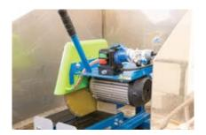
Water-cooled tile saw used for cutting large rock samples.
