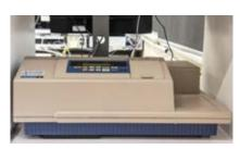
With cuvette and plate reading capability for UV-Vis absorption and fluorescence.
