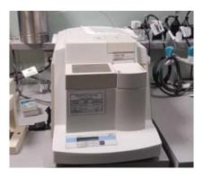
The DCS-60 differential scanning calorimeter is an efficient and powerful tool for quick determination of specific heat and enthalpy change accompanying the primary or secondary phase transition of a substance.
