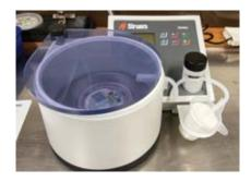
Vacuum impregnation unit that uses compressed air for the impregnation of porous samples and materials. Special mounting cup holders allow for the preparation of multiple specimens at the same time.
