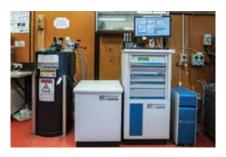
This PPMS is capable of measuring a broad range of magnetic, thermodynamic, and electrical transport properties at temperatures from 2–400 K and in magnetic fields up to 7 T. Properties that can be measured include electrical resistivity, Hall effect, thermal conductivity, and magnetisation. It can also be configured for custom user experiments.
