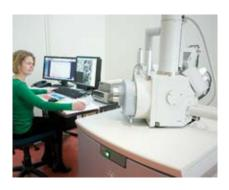
The FEI Nova is a high-resolution, field emission gun SEM (FEG-SEM), with excellent imaging and analytical performance. It is equipped with an energy dispersive X-ray spectrometer (EDS or EDXS) for elemental analysis and an electron backscatter diffractometer (EBSD) for crystal orientation mapping.
