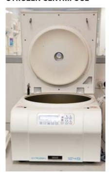
A multi-purpose large-capacity centrifuge with a maximum speed of 12,000 rpm with high capacity and a large assortment of rotors.
