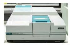
The Cary 100 Bio UV-Vis is a powerful double-beam spectrophotometer capable of quickly acquiring data in the spectral range from 200 to 900 nm.
