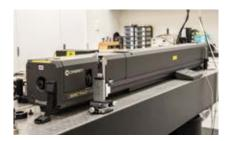
This laser provides the ultimate in highpower ion laser performance, combined with extraordinary ease-of-use. A single digital remote module gives you access and control of all critical laser functions such as wavelength acquisition and tuning, automated TEMOO-acquiring shutter, extra-cavity shutter, system monitoring, and diagnostics.
