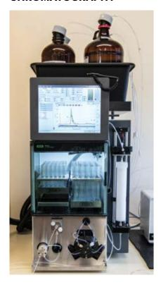
Multiple Buchi automated flash chromatography systems for automated and quick isolation of compounds using UV and ELSD detection.
