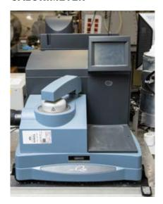
The DSC Q100 Differential Scanning Calorimeter is an efficient and powerful tool for quick determination of specific heat and enthalpy change accompanying the primary or secondary phase transition of a substance.
