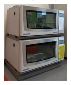
Ferrier has six shaking incubators (one dark and five refrigerated) used to grow biological cultures.
