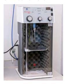
The Omni Sonic Ruptor 4000 offers precision engineering with all the features necessary to create a total system for ultrasonic disruption. Popular applications include nanoparticle dispersion, creating emulsions, cell disruption, and homogenisation. The Sonic Ruptor 4000 is capable of creating an emulsion down to 1/100 of a micron.
