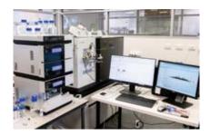
The Thermo Scientific Orbitrap Fusion Lumos Tribrid Mass Spectrometer is an advanced performance mass spectrometry system that can be upgraded to even higher resolution (1 M), additional dissociation capabilities (UVPD and ETD), and a unique internal calibration (IC). Excels at the most challenging of applications, including low-level PTM analysis, multiplexed relative quantitation using isobaric tags, intact protein characterisation, as well as MSn analysis of small molecules.
