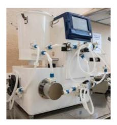
Multi-litre molecular sizing and dialysis/ ultra filtration. A semi-automated tangential flow filtration/cross flow filtration system for concentration and diafiltration as well as cell harvest and clarification.
