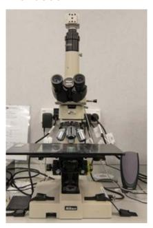
This Nikon optical microscope with digital camera is used to inspect samples during processing runs.
