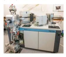
Thermal lonisation mass spectrometer for high-precision isotope ratio measurement in geological samples.
