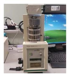
The TGA-50 is optimally applicable to the measurement of adsorbed water, water of crystallisation and residual solvent, the thermal stability of substances, and solid (liquid) to gas and gas to solid (liquid) phase changes in decomposition and oxidation reactions.
