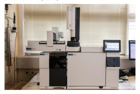
Separation and mass identification of volatile chemical compounds in samples.
