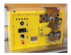
Magnetic susceptibility separator utilising paramagnetic and diamagnetic properties of minerals. Suitable for large (1–2 kg) sample volumes.
