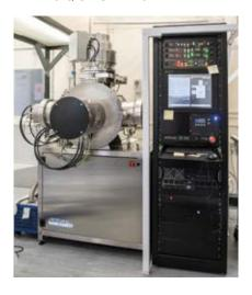
lon beam etching system for patterning thin film devices.
