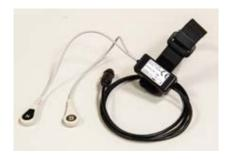
This Galvanic Skin Response (GSR) sensor connects to the expansion port on the Equivital SEM to enable recording of GSR signals. It consists of a small box that can fit inside the equivital sensor belt or be worn on the wrist as well as short leads terminating in standard 'snap lead' connectors suitable for use with the MLA1010 disposable electrodes.
