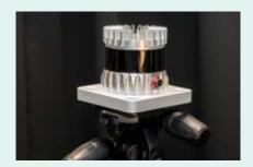
This laser environment scanner is used to measure distances by illuminating the target with laser light and measuring the reflection with a sensor. These measurements can then be used to make digital 3D representations.
