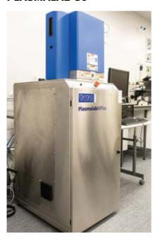
Reactive ion etching is a common process in microelectronics to carve patterns into silicon or any other substrate material. At present, the School has Ar, O², and SF6 gas for etching. Whether your material can be etched with this system will depend on the gases available and the selectivity between your substrate material and any standard mask. Determining the etch recipe takes time, so users should add this to their expected experimental time.
