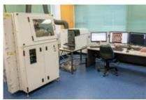
Quadrupole mass spectrometer for trace element analysis by solution or coupled to the Resonetics Laser Ablation system.
