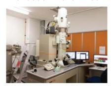
The JEOL JEM-2100F is a 200 kV field emission transmission electron microscope (TEM) that combines high spatial resolution and analytical performance with an easy to use operation system, ideal for multipurpose operation.
