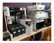
Preparative-scale chromatography enabling the isolation, purification, and collection of target compounds.
