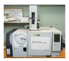
The GCMS-QP2010 is a bench-top type gas chromatograph/mass spectrometer intended for high-precision GC/MS analysis. It enables mass spectrum measurement for qualitative analysis or identification of unknowns and Selected Ion Monitoring (SIM) measurement for quantitation of trace constituents.
