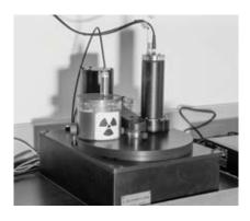
The RISO Reader is a luminescence dating instrument that contains a 48-position automated sample changer, a beta radiation source, and stimulation devices for thermoluminescence and optically stimulated luminescence (infrared, green, and blue light).
