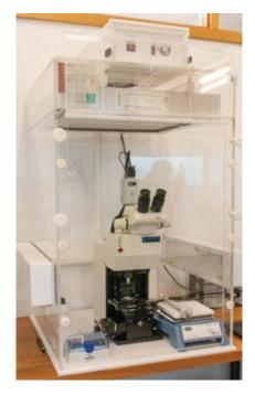
Micromilling device designed for highresolution milling to recover sample powders for chemical and isotopic analysis.
