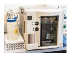
Grain size analyser using electrical impedence through a suspended sample (i.e. Coulter Principle: Electrical Sensing Zone (ESZ)).
