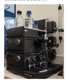
Low pressure (low flow rate) semipreparative liquid chromatography system with fraction collector suitable for separating compounds (mg scale) on size exclusion, anion-exchange, or other columns.
