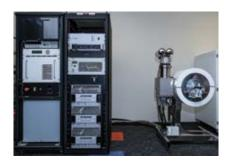
Capable of imaging up to 100 mm diameter samples. Single TX/RX RF coil. MR Solutions spectrometer and GUI with standard MRI pulse sequences.
