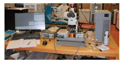
Polarising light microscope with an electromagnet for measuring magneto-optical effects.
