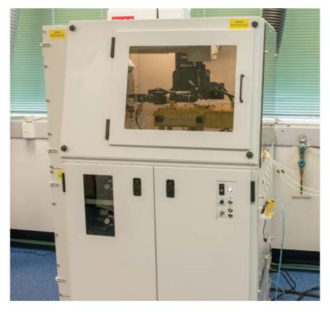
193 nm excimer laser ablation system with Laurin Technic S155 Sample cell and GeoStar software for in-situ trace element analysis of a range of solid materials.
