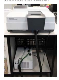
UV-Vis Spectrophotometer with temperature controller.
