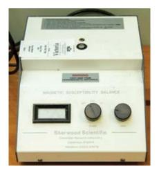
Used to determine the magnetic properties of materials.
