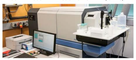
Single collector, double-focusing magnetic-sector field mass spectrometer for trace element and isotopic analysis. This instrument can be linked to the Resonetics laser ablation system for the analysis of solid materials. This instrument can also be used in solution mode where samples are digested and diluted appropriately in solution.
