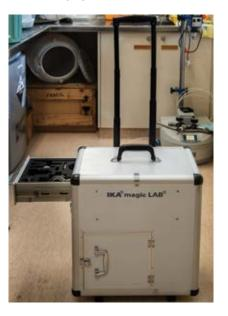
Small-scale, portable, laboratory machine designed for mixing, dispersing, wet milling, and incorporation of powders into liquids.
