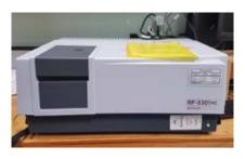
The RF-5301PC allows high-sensitivity analysis to be carried out, based on a unique optical system that involves a highly efficient blazed holographic grating as well as a low-noise circuitry that includes a digital filter.
