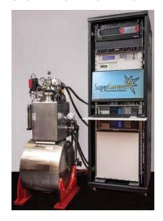
Used to accurately determine the critical surface of highly anisotropic superconductors. The Robinson Research Institute, in conjunction with HTS-110 Ltd, has designed and built the only commercially available system specifically designed for the real-world transport characterisation of superconducting wires under the actual conditions of relevance to specific applications. It accurately determines in detail the critical surface of highly anisotropic superconductors.
