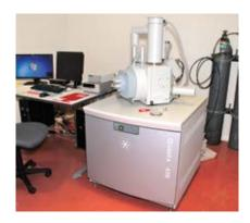
The FEI Quanta is the Institute's workhorse instrument and can operate in high, low, and environmental (or ESEM) vacuum modes. It is equipped with an energy dispersive X-ray spectrometer (EDS or EDXS) for the elemental analysis of materials.
