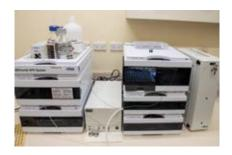
Specialist analytical HPLC for size determination of oligo- and polymeric structures.
