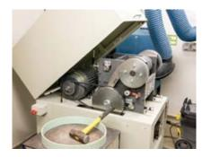
This crusher is a double-acting fine jaw crusher. Its design includes top- and bottom-driven moving jaws, enabling the maximum amount of crushing in a single pass. It takes lump sizes of up to 150 mm pieces and crushes them to 10 mm or less. Jaws can hold up to 20 kg of sample in one load.
