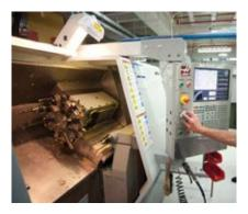
HAAS CNC Metal Lathe (SL-20) with auto-multi-tool changer. Uses VisualMill/VisualCam for toolpaths.
