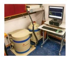
The gamma-ray spectrometer is an instrument for measuring the distribution (or spectrum) of the intensity of gamma radiation versus the energy of each photon. It is a quick and non-destructive analytical technique that can be used to identify various radioactive isotopes in a sample.
