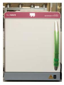
Milestone's flexiWAVE overcomes the limitation of conventional microwave synthesis devices, as it consists of a single microwave platform that, in combination with specific accessories, allows chemists to perform classic glassware and high-pressure synthesis, as well as solid-phase reactions.
