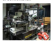
This triple additive/subtractive high resolution Raman spectrometer facility (Jobin-Yvon T64000) is coupled to a confocal Raman microscope and five different lasers: argon, krypton, helium-cadmium, helium-neon, and NIR-solid state. The spectrometer has both a nitrogen-cooled CCD detector and a photomultiplier (GaAs-cathode). It is also possible to access (Raman) mapping stages and low temperature conditions—down to 77 K for the microscope and 8 K in the separate closed cycle cryostat.
