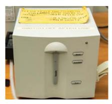
The Agilent 8453 UV-Vis instrument is a simple but powerful diode-array spectrophotometer capable of quickly acquiring data in the spectral range from 190 to 1100 nm.
