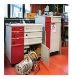
The MPMS measures magnetic properties of materials from 1.9–400 K in up to 7 Tesla magnetic field.
