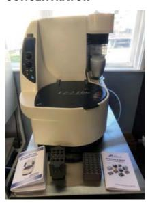
Sample concentration/solvent removal under reduced pressure and centrifugal force
