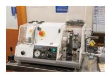
For use in the preparation of petrogeogical thin section slides. The instrument is used to trim samples from bonded glass slides and grind these down to a desired thickness before the final polishing process.
