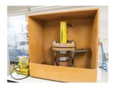
Hydraulic press used for breaking up large rock samples into smaller, more manageable sizes.
