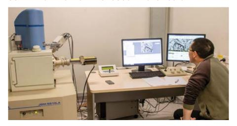
This microscope offers seamless transition between imaging and analysis. A general-purpose, thermal type SEM to meet the needs of a wide range of users, as standard recipes simplify the setting procedures. The standard 5-axis motor stage makes it easy to locate the area of interest.
