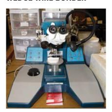
Manual mode operation wire bonder for attaching wires to make electrical measurements.
