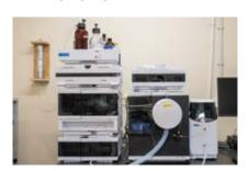
For reaction monitoring, separation, and detection of chemical compounds in a sample to determine purity and composition. Detectors include UV and ELSD.
