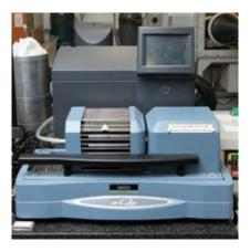
The Q600 provides simultaneous measurement of weight change (TGA) and true differential heat flow (DSC) on the same sample from ambient to 1500°C. It features a field-proven horizontal dual beam design with automatic beam growth compensation, and the ability to analyse two TGA samples simultaneously. DSC heat flow data is dynamically normalised using the instantaneous sample weight at any given temperature.
