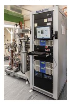
The six-target Kurt J Lesker CMS-18 thin film sputtering system is a state-of-the-art thin film deposition system for advanced materials research and development.
