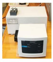
The Agilent 8454 UV-Vis instrument is a simple but powerful diode-array spectrophotometer capable of quickly acquiring data in the spectral range from 190 to 1100 nm.
