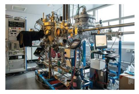
The Riber molecular beam epitaxy system is capable of growing epitaxial thin films of extremely high crystalline quality and with atomic level thickness control. Multiple deposition sources allow growth of alloys and multi-layered samples. The system is presently configured for the growth of nitrides.
