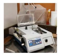
Gravity-fed diamond-bladed saw with variable speed (50–900 RPM) for cutting rock and mineral samples. Particularly suitable for delicate/fragile samples.
