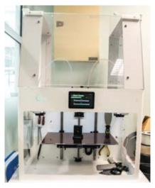
The Craftbot Flow IDEX printer is a duel independent 3D printing system capable of printing using a range of materials up to 300°C. It has a build volume of  $425 \times 250 \times 250$  with a layer resolution of 50 µm.
