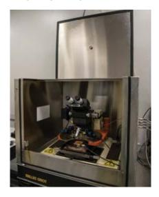
The probe station is set up with four highprecision Ti probes on micromanipulators and is housed in a custom-made Faraday box with a high-quality co-axial cable running to the micromanipulator. The probe station is equipped with a vacuum chuck and objective lenses of various magnification for maximum flexibility. Users are encouraged to buy their own tips for non-standard samples.
