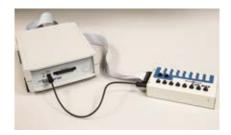
This amplifier is a bipolar amplifier that can be used to record EMG, ECG, EOG, and polygraphic channels such as GSR, acceleration, temperature, and blood pulse with an extremely compact design.
