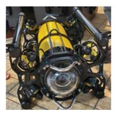
Lightweight Remotely Operated Vehicle (ROV) that can be easily deployed and operated with a small crew of two form virtually any small boat. At 23 kgs, it is easy to launch and recover by hand and can safely operate to depths of up to 500 metres.
