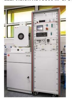
The HHV sputter coater by Ezzi Vision has a single-source RF magnetron sputter deposition target. The system is capable of depositing both metals and dielectrics, including Ti, Ag, Ni, SiO<sup>2</sup>, and ZnO at present. The system comes equipped with an INFICON rate deposition controller for high accuracy of film thicknesses. Frequent users will be required to provide their own 3-inch diameter source material.
