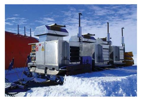
The boilers and generators to operate the hot water drill system.
