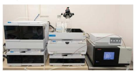
Separation and detection of chemical compounds in a sample to determine sample purity and composition. Detectors include UV and charged aerosol detector (CAD).
