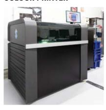
Stratasys J850 multi-material 3D colour/ VOXEL Printer is a polymer 3D printer able to print flexible and rigid multi-colour prints, down to a VOXEL level of detail. A VOXEL is like a PIXEL but 3D.
