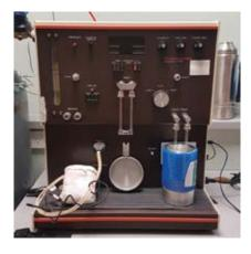
The FlowSorb II measures surface area using the flowing gas method, which involves the continuous flow of an adsorptive and inert gas mixture over the sample at atmospheric pressure.
