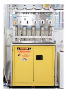
The PureSolv MD5 solvent purification system allows easy access to anhydrous solvent by multiple users. Its multi-way valve design is the most efficient and safest air-free dispensing system on the market today.
