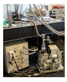
This closed cycle cryostat is capable of operating from above room temperature to ~4 K. It is equipped with viewports that enable optical measurements from the infrared to the UV, and electrical feedthroughs allowing measurement of the electrical resistance of samples from milliOhms to hundreds of gigaOhms.
