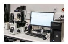
The MMI CellCut facilitates precise and contamination-free dissection of cell clusters, single cells, or subcellular compartments from various types of tissues including fresh frozen, paraffin embedded and archived slides, cytospins, smears, and even living cells.
