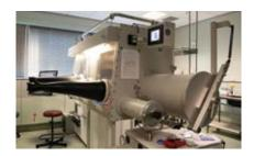
Inert-atmosphere gloveboxes is available for device fabrication. One has spin coater for thin film. One has a thermal evaporator chamber for the deposition of metal oxides, organics, and electrodes.
