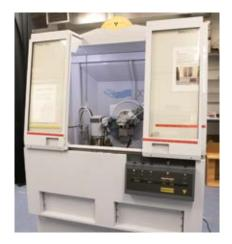
Used for the analysis of morphology, mechanical properties, content, and structure of materials. Services include high-resolution powder diffraction, phase identification and quantitative phase analysis, analysis of thin films and coatings, crystallite size and strain determination, kinetic and non-ambient experiments.
