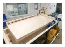
This heavy/dense mineral separator is typically used for the following applications: Technical research—assessment of gravity processes, geochronology studies, characterisation of heavy minerals, recovery of precious metals (e.g., gold rooms), separation in synthetic diamond manufacture, and quality control—silica sand processing/ glass-making industry.
