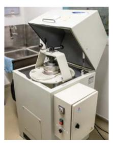
This ring mill is used for coarse pulverising of large rock samples for mineral separation such as Zircon dating, preparing samples for on-stream analysis, dry, or slurries. Low maintenance and easy to clean, this ring mill features a continuous flow-through operation with built-in ducting of cyclone with external connection to dust extraction systems for cleaning the head. Sample bin holds up to 10 kg. Quiet operation—less than 85 dB.
