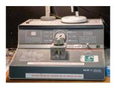
The procedure of critical point drying is an efficient method for drying delicate samples. It preserves the surface structure of a specimen which could otherwise be damaged due to surface tension when changing from the liquid to gaseous state.
