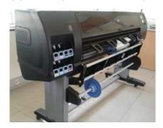
The Technical Resource Centre has two HP6800 series wide format 8-colour plotters, and a Seilka LPT1020 wide format colour scanner, used for architectural and design processes, capable of scanning large format (A0) colour images and printing large format (A0 up to 4 m  $\times$  1.5 m) colour prints on various papers.
