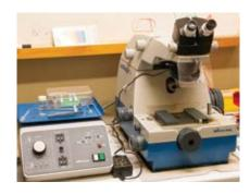
Ultramicrotome can be used to cut specimens into extremely thin slices, called ultra-thin sections, that can be studied and documented at different magnifications in a transmission electron microscope (TEM).
