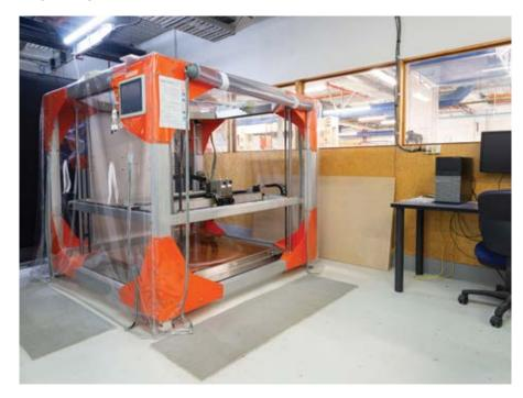
Large FDM 3D printer (BigRep ONE v3). Large 1  $\rm m^3$  print volume Fused Deposition Modelling 3D printer.
