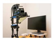
This eye tracker is a system for tracking eye movements, fixations, and pupil dilation in relation to events that occur on a computer monitor.
