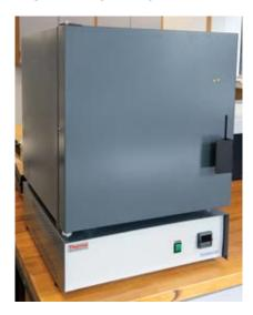
Large capacity muffle furnace suitable for gravimetric analysis, sintering, quantitative analysis and heat treatment.
