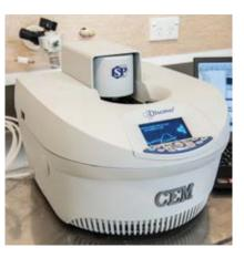
Synthesis equipment for conducting organic synthesis reaction under microwave conditions.
