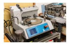
For use in the precision lapping of petrological and mineralogical samples, specifically for petrographic thin section slide preparation.
