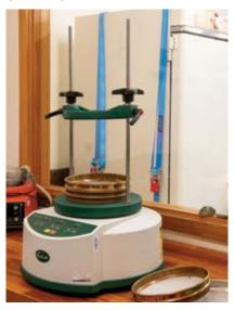
Test sieve shaker with 3D sieving motion, suitable for up to 8 full height/16 half height sieves.
