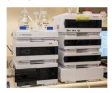
Separation and detection of chemical compounds in a sample to determine purity and composition. Detectors include UV, fluorescence, and refractive index (RI).
