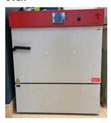
This oven is used in temperature and humidity experiments, cell culture, and enzyme experiments.
