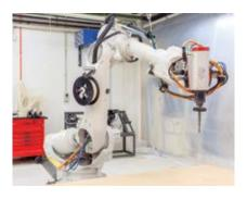
ABB Robotic Arm (large fixed-installation IRB 6700–200/ 2.6 m) with milling, gripper heads, fencing, and tool changer. This is used to investigate full-scale additive and subtractive manufacture, and other programmatic CNC controlled applications using Robot Studio and other programs such as Rhino/Grasshopper.
