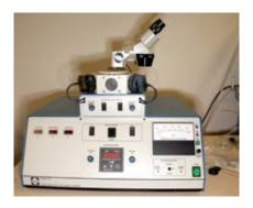
Equipment to support SEM and TEM work includes a carbon coater, metal coater, and a Gatan Precision Ion Polishing System (PIPS).
