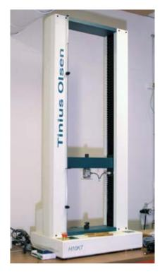
Tests the resistance of a material to breaking under tension.
