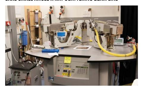
Small-angle X-ray scattering (SAXS) is a small-angle scattering technique by which nanoscale density differences in a sample can be quantified. In the case of biological macromolecules such as proteins, the advantage of SAXS over crystallography is that a crystalline sample is not needed.
