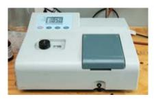
The 722N UV-VIS spectrophotometer adopts advanced proportional double beam optical system and low noise circuit design, with excellent reliability and stability. It can meet the needs of daily analysis, scientific research, and other applications.
