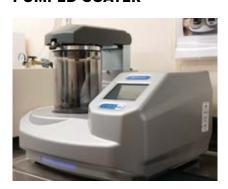
The Q150T Plus has been optimally developed for use with a turbomolecular pump, which offers a lower vacuum down to  $5 \times 10-5$  mbar. This allows the sputtering of oxidising metals, which have a lower grain size ideal for high-resolution imaging. Likewise, lower scattering enables the development of high-purity, amorphous carbon films with a high density.
