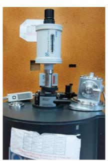
The VSM measures magnetic properties of materials in up to 1 Tesla magnetic field and from 300 to 20 K.
