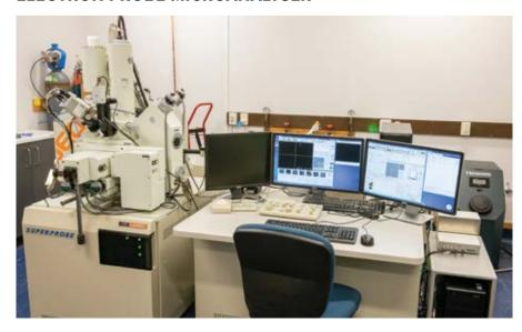
JEOL JXA-8230 SuperProbe Electron Probe Microanalyser, with 5 wavelength dispersive X-ray spectrometers (WDS), an energy dispersive X-ray spectrometer (EDS) analyser featuring spectral imaging, a JEOL xCLent 3 cathodoluminescence (CL) spectrometer, and highly sensitive detectors for acquisition of backscattered electron (BSE) and secondary electron (SEI) images.
