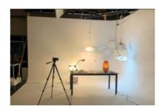
A 3D cyclorama approximately 4 m x 3 m x 3 m. This is a white cyclorama allowing colour keying of still and video shots, for subsequent video editing/compositing. It is installed with spot lights and washlights preconfigured for users allowing for most requirements—thus needing no specialist support.
