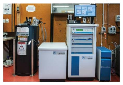
The PPMS measures magnetic, magnetotransport, and thermoelectric properties of materials from 1.9-1000~K in up to 9~Tesla magnetic field.
