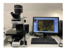
BX63 motorised upright microscope which does brightfield, DIC, and fluorescence. Can also do multi imaging z stacks.
