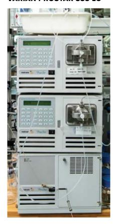
The Varian ProStar 335 is a HPLC photodiode array detector that can simultaneously detect the absorbance of compounds in the flowcell at wavelengths from 190 to 950 nm.
