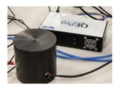
The QE Pro is a high sensitivity spectrometer with low stray light performance. It is ideal for a wide range of low light level applications such as fluorescence, DNA sequencing, and Raman analysis.
