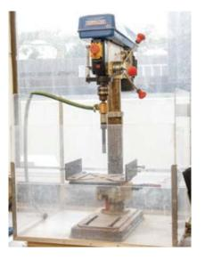
For use in diamond drilling paleomagnetic core samples.
