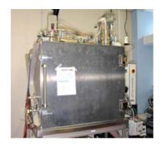
For testing of coils, magnets, or other assemblies. Internal dimensions are 1 x 1 x 1 m. Comes complete with roughing and turbo pumps, and single stage cryocooler if required.
