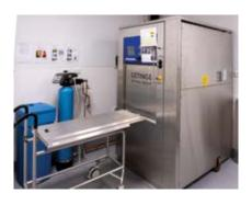
Autoclave for processing of laboratory waste.
