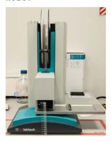
Robot for protein crystallisation condition screening.
