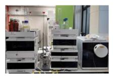
Separation and detection of chemical compounds in a sample to determine sample purification. Detectors include UV and mass spectrometry.
