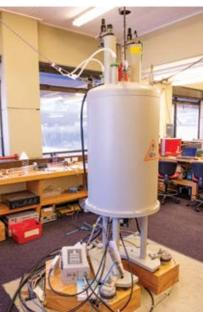
Two Bruker machines—400 MHz Bruker Avance II. Used for studying the rheology and diffusion of soft materials or the flow dynamics of liquids in porous media.
