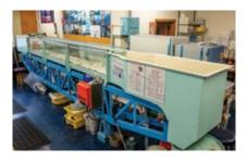
Built in 1978, 'The Flume' mechanical stream flow simulator is used to simulate and observe particle motion, bedforms and flow characteristics. Stream flow channel: 7 m long, 0.4 m wide; max depth 0.3 m; max velocity 0.8 m/s. Slope of channel can be hydraulically tilted downstream to 1.2 m. Silica sand bed (modal particle size 180  $\mu$ m) with contrasting iron sand (used to show internal structure of bedforms).
