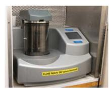
The Q150T Plus enables the sputtering of oxidising metals, which have a lower grain size suitable for high-resolution imaging. Similarly, lower scattering allows for high purity, amorphous carbon films of high density.
