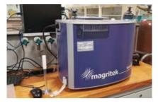
The Spinsolve benchtop NMR is a compact benchtop NMR spectrometer used for 31P spectra. The high NMR sensitivity, simple spectra, and large chemical shift range of 31P and the lack of common background signals (such as solvent signals) make 31P NMR suitable for routine purity assessment and reaction monitoring.
