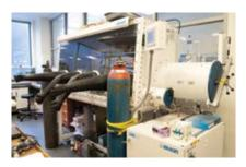
Braun glovebox systems are operated using a closed loop circulation method, providing the user with a non-reactive atmosphere.
