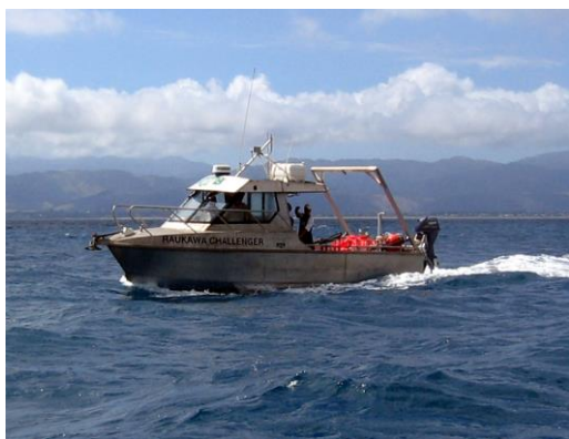
Figure 6. VUCEL Research vessel, Raukawa Challenger , 8.5m aluminium tri-hull
